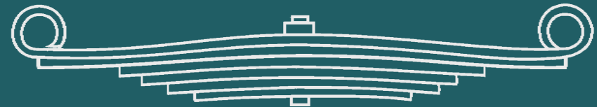
Extra Leaf Added - Same Length as Main Leaf Improperly Stepped Spring
